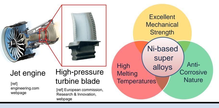
A superalloy contains rare (scarce) and expensive "refractory metals" such as Rhenium (Re), Tungsten (W) and Tantalum (Ta) for their high-temperature strength.
