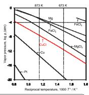
Reaction temperature was determined at 873 K CuCl<sub>2</sub> and CuCl were selected for the chlorinating agent.
