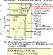
$\rightarrow \text{FeCl}_{x}(g) \uparrow + \text{H}_{2}\text{O}(g)$   $\text{FeO}_{x} (\text{FeTiO}_{x}, s) + \text{CaCl}_{2}(l)$ → FeCl<sub>x</sub>(g) ↑ + <u>CaO (CaTiO<sub>x</sub>,s)</u> a<sub>CaO</sub> << 1
