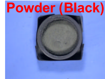
Residue in the graphite Crucible after heating (C)
