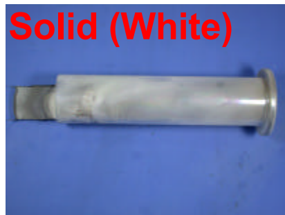
Deposit on the surface of the NaOH gas trap (A)
